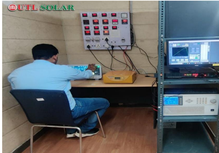
Off grid inverter testing set up
